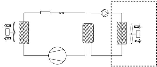
The cooling system created is placed in the lower part of the vending machine in an area well ventilated by the condenser fan, and even if there was a leakage of R290 from the primary circuit, it would not be entering in an area confined inside the refrigerated cell.
