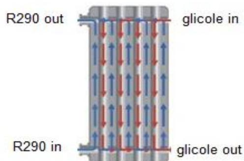
The cooled glycol in the plate exchanger is then sent through a circulation pump, in a finned pack exchanger positioned inside the cell of the vending machine for the products stored at a controlled temperature.
